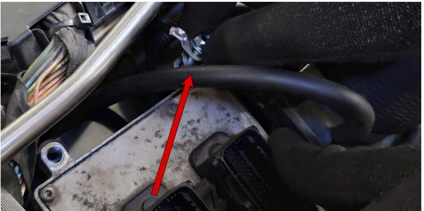
11. Install M6x20 screw (marked green) in upper right hole through ground cables connectors. Do not tighten yet.
